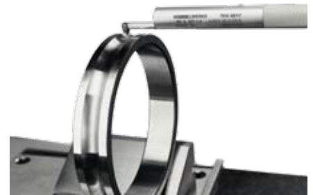
TKK 50 skidded for concave and convex surfaces
