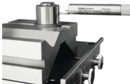
TKO 50 skidded for small diameter bores (2mm)
